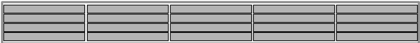
The figure above shows a 1U system with twenty (20) front loading E3 thin devices. Using a device pitch of 9.3mm, a 2U platform can support a maximum of between forty-four (44) and forty-six (46) front loading E3 devices depending on the 2U chassis mechanical structure. Actual implementations will vary based on thermal and workload targets as described below.
